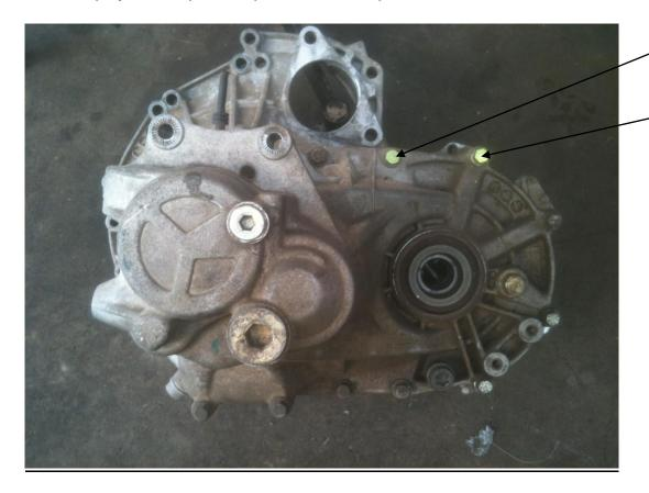
The two bolts shown need to be drilled 2.5 mm dia to take an MG Trophy seal.
