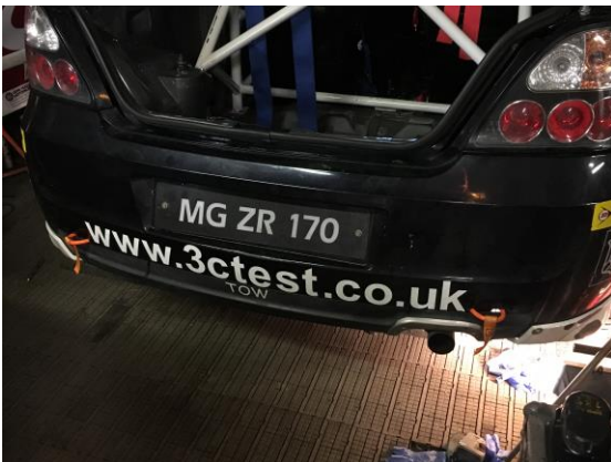
Fig 7 no more than 25mm protrusion
